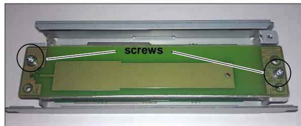
4. Attach the antenna and secure with 2 screws, the proper alignment shown in the figure above.
