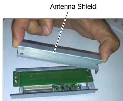
2. Remove the screw holding the antenna shield
