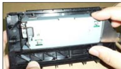
5. Pass the ground wire through the hole in the sheet metal as shown in the photo , and secure it with screws (PT-3x6).
