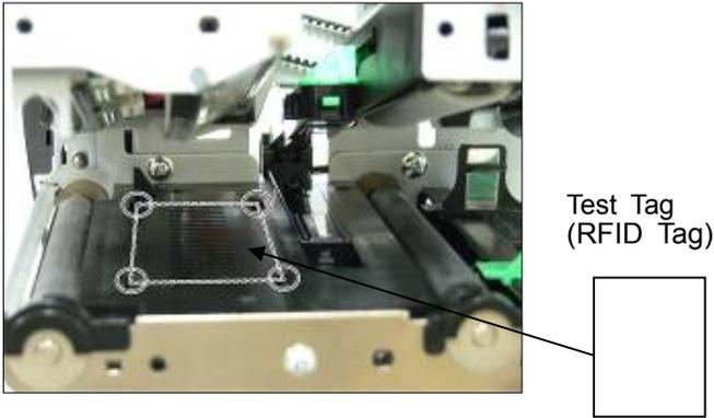
To select [TEST] and pushing [ENTER]key. and pushing [ENTER]key by selecting 「ID READ」, and execute ID READ test.. After that, the read ID appear on the display
