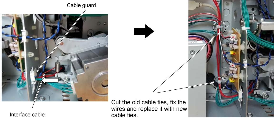
7. Arrange the cables properly and secure it on the cable clamp as shown below.
