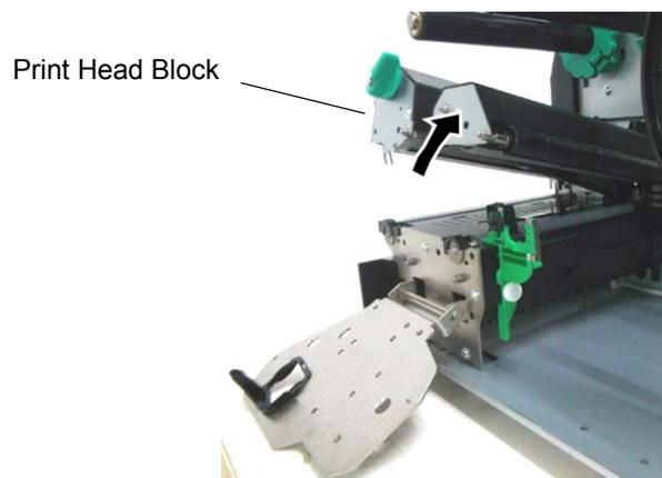
3. To release the hook, Insert the tip of a thin tool into the square hole, remove the platen holder cover and remove the Strip plate.
