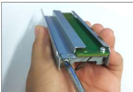
1. Remove the screws that secure the antenna shield.
