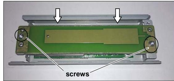
2. Move the antenna in the middle position and observe proper alignment as shown in the figure above. Attach the two screws back with the new
