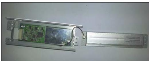
3. Re- connect the black wire to the antenna as shown in figure above
