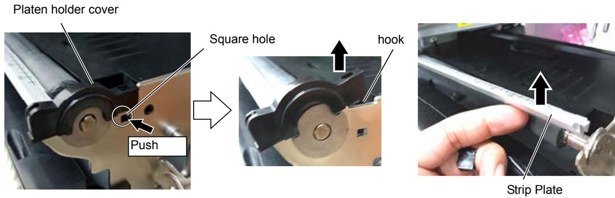
4. Install the RFID paper guide and return the platen holder cover to the original position.
