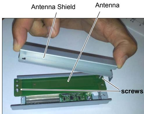
1. Remove the antenna shield as per Step 1 to 2 of Front Position (Antenna Shield Disable), and remove 2 screws as shown.
