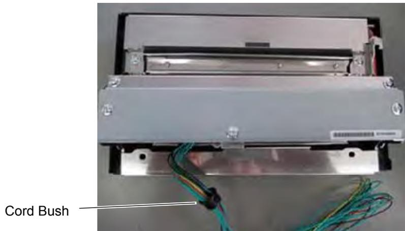
8. Attach the Cable Clamp to the printer base.
