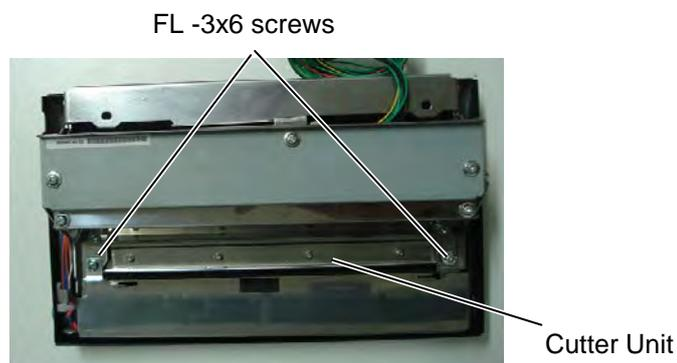
6. Apply FLOIL HTM-308 to the cutter unit using a soft cloth.
