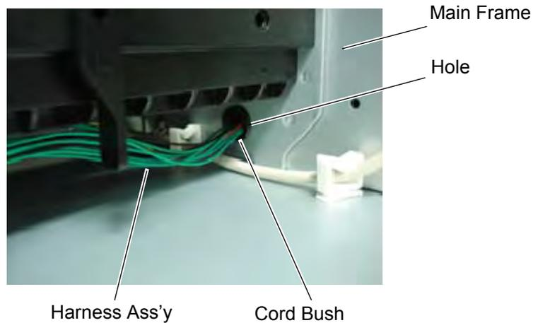
**NOTE:** Make sure the wires will not touch or obstruct any moving parts.
