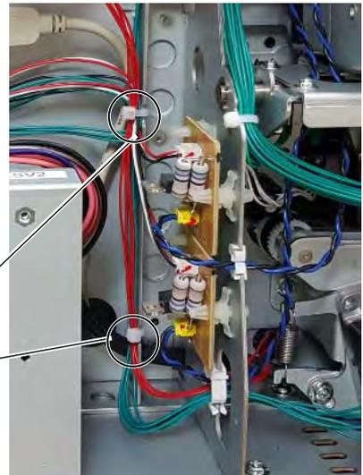
Cut the old cable ties and fasten the cables together with the interface cable with new cable ties.
