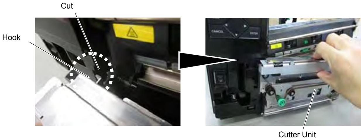
10. Secure the right side of the Cutter Unit with the ST-3x6 screw.
