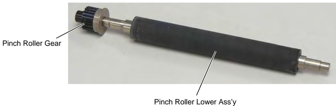
2. When reassembling, make sure that the pinch roller lower ass'y is attached correctly. Also, make sure that the pinch roller holder cover is fixed with the hook.
