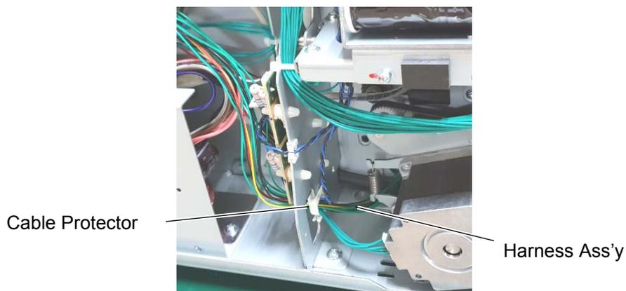
2. Fasten the Harness Ass'y with the Cable Clamp.
