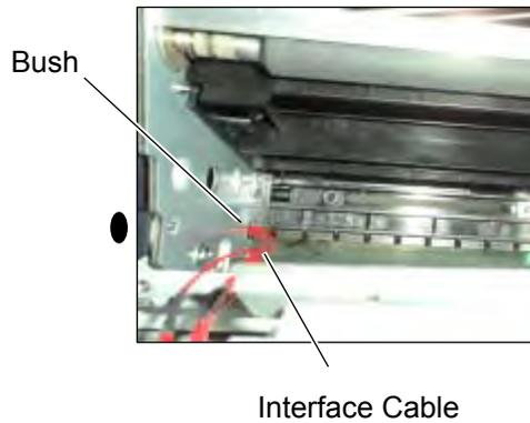
4. Fit the RFID module to the bottom of the Platen Holder Block as shown below.
