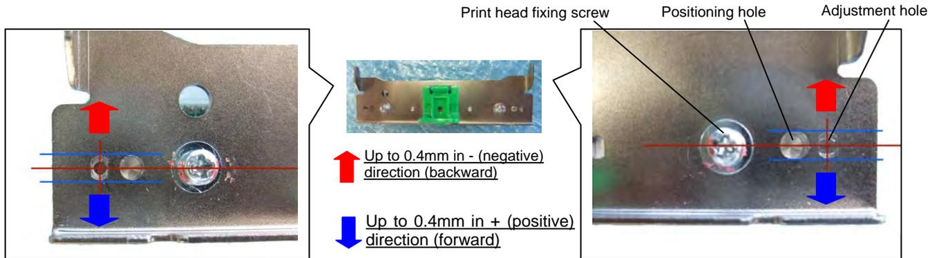
7) When the best position is determined, tighten the print head fixing screws.
