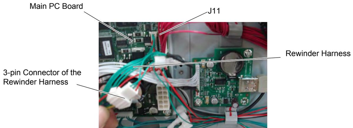
15. Fasten the harness of the 4-pin Connector of the Rewinder Harness with Cable Clamp and Cable Protector. And then insert the 4-pin Connector of the Rewinder Harness into the hole of the main frame.
