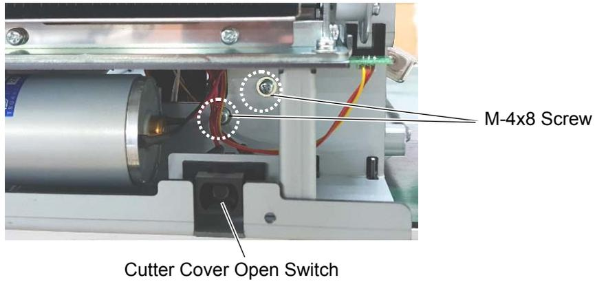
7. Attach the Cutter Cover to the Cutter Unit with the two screws so that the tab of the Cutter Cover turns on the Cutter Cover Open Switch.
