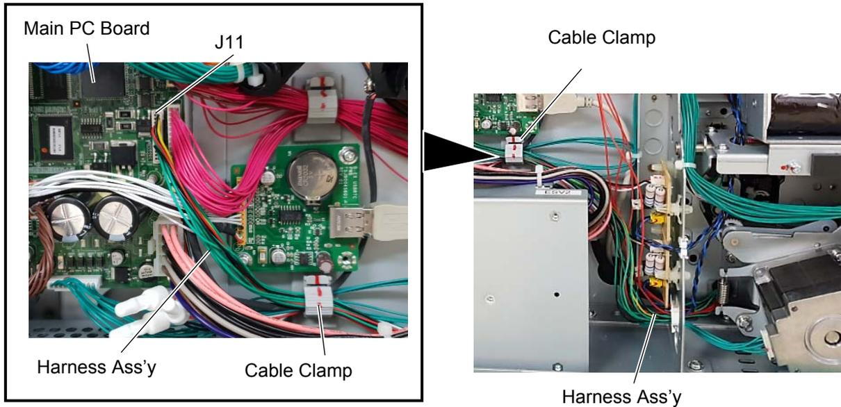
**NOTE:** Wind the Harness Ass'y around the cable clamp if the harness is too long.
