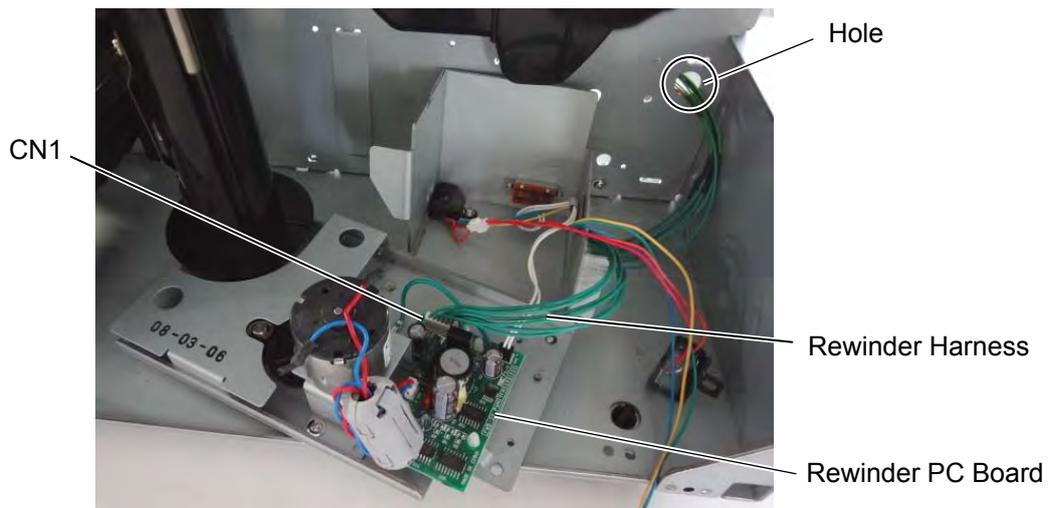
6. Re-attach the Rewinder Motor Cover with the two screws, and pass the Rewind Full Sensor Harness to the other side of the Main Frame through the hole.
