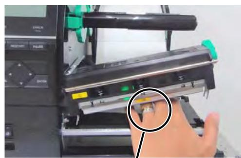
Care must be taken not to allow a metal object like a ring to touch the print head edge.
