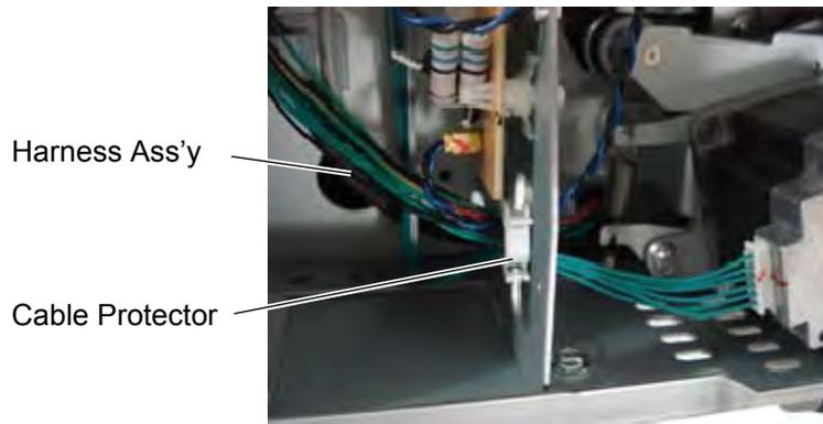
2. Fasten the Harness Ass'y with the Cable Clamp.
