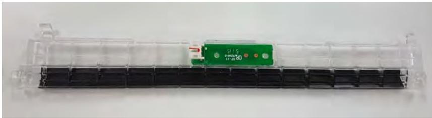
**NOTE:** After replacing the ribbon end sensor, refer to Section 5.7 to adjust the sensor level for the ribbon to be used
