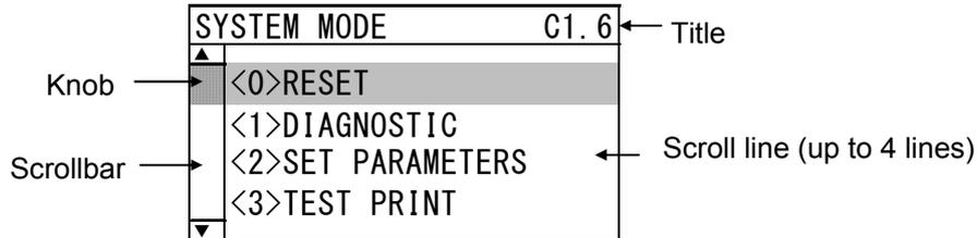
The knob appears on the scrollbar when the number of scroll lines is over 4 lines.
