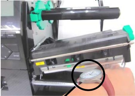
Care must be taken not to allow the metal or glass part of a watch to touch the print head edge.
