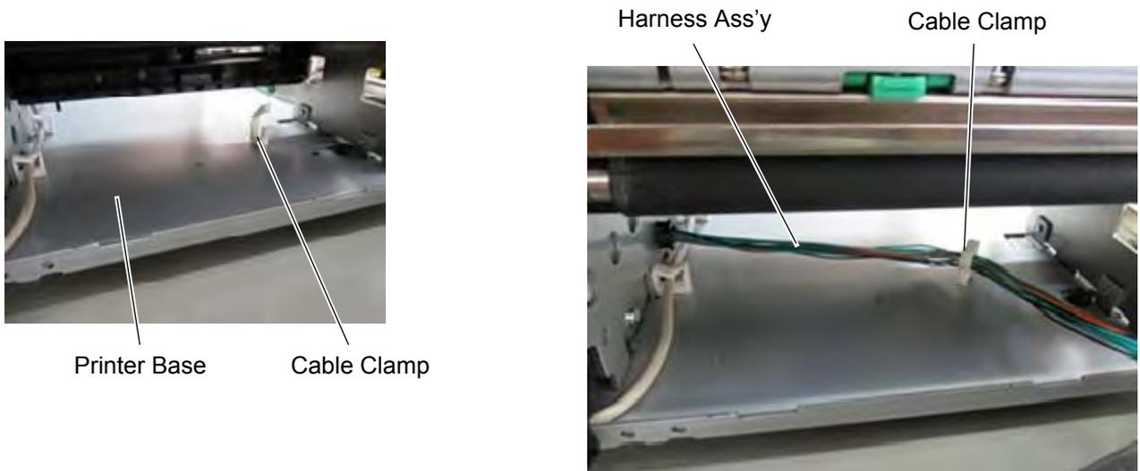
**NOTE:** Make sure the wires will not touch or obstruct any moving parts.
