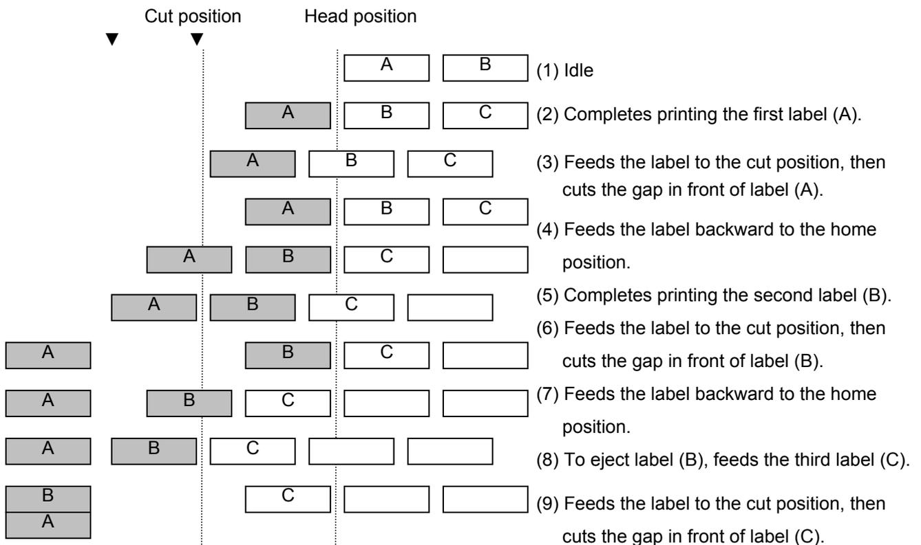
3. Procedure for label having less than the min. label pitch for each issue speed when the rotary cutter is used
