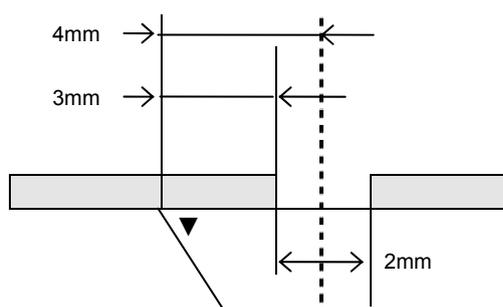
Printing in strip issue mode is stopped at the position where the distance from the middle point of the gap between labels to the end of the strip shaft is 4 mm, since the gap between labels is assumed to be 2 mm. When the print stop position is not proper due to a greater gap, the print stop position should be adjusted using the strip position fine adjust function.
