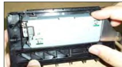
5. Pass the ground wire through the hole in the sheet metal as shown in the photo, and secure it with screws (PT-3x6).
