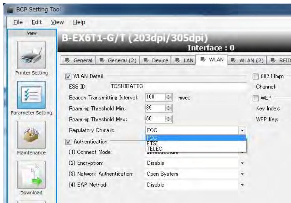
When using a printer outside the "FCC" area, please perform the following key operation and activate the "Regulatory Domain" field.
