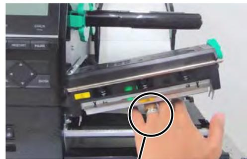
Care must be taken not to allow a metal object like a ring to touch the print head edge.
