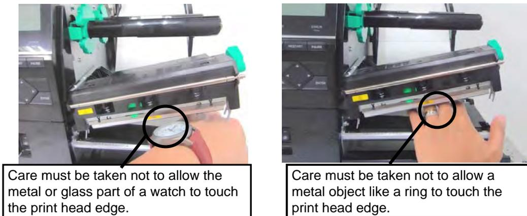
Since the print head element can be easily damaged by shock, please treat it carefully by not hitting a hard object against it.
