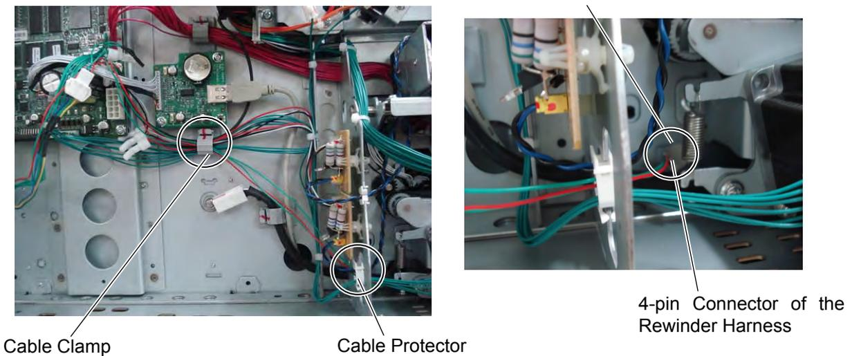
16. Fit the Cord Bush to the 4-pin Connector of the Rewinder Harness, in the orientation shown below. Then fit the Cord Bush into the hole.
