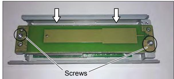
2. Move the antenna in the middle position and observe proper alignment as shown in the figure above. Attach the two screws back with the new antenna position.
