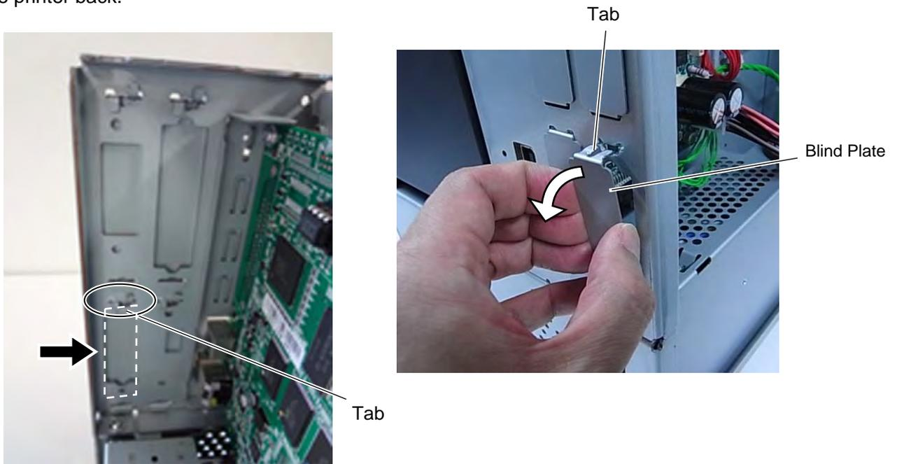
5. Fit the Expansion I/O Connector of the Expansion I/O Board into the slot from the inside, and secure it with the two M-3x6 screws from the outside, as shown below.
