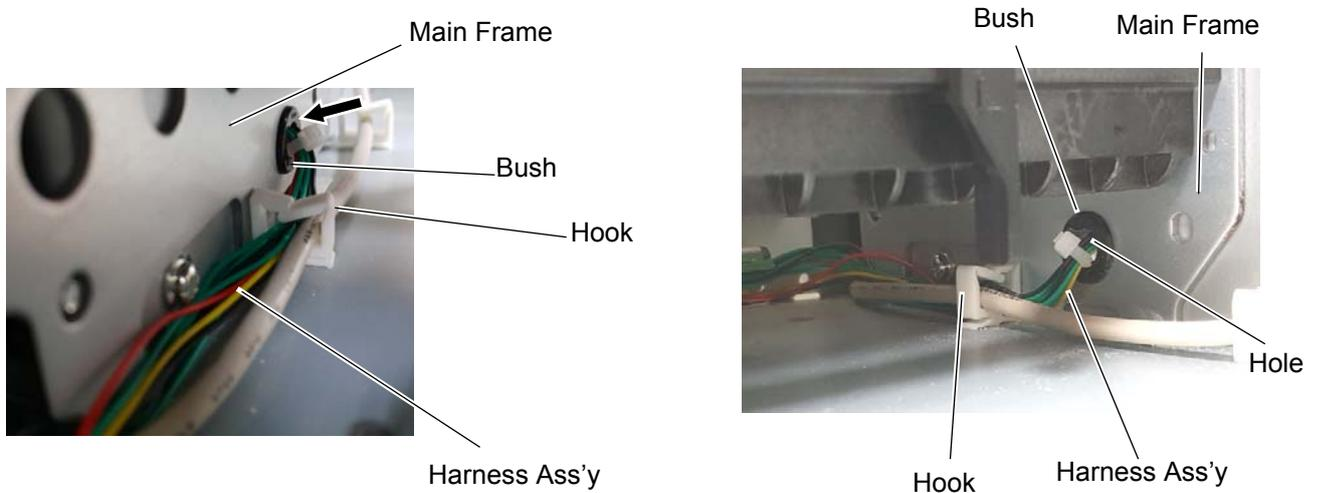
**NOTE:** Make sure the wires will not touch or obstruct any moving parts.
