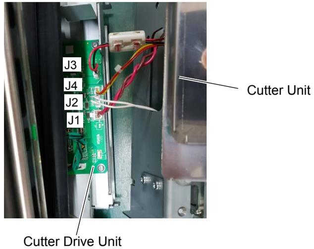
5. Place the hook at the left side of the Cutter Unit on the cut in the printer main frame. Fit the tab of the Cutter Drive Unit into the slit in the Cutter Unit.
