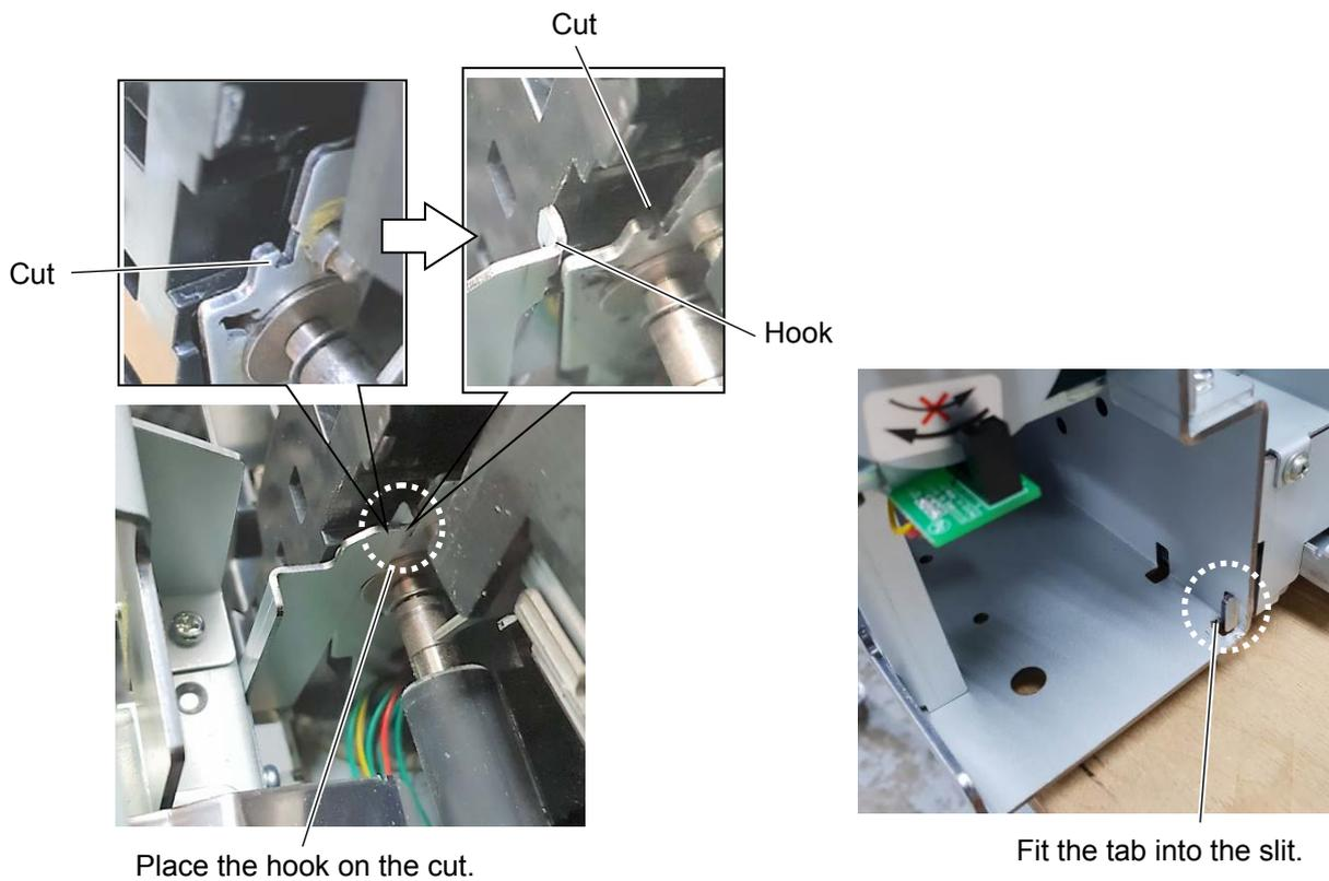
6. Secure the Cutter Unit with the M-4x8 screws.
