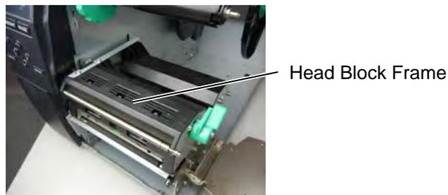
5. When replacing parts or performing maintenance on the printer, be careful not to damage the print head with a hard object like a watch or a ring.
