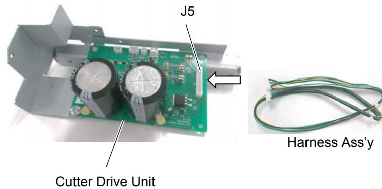
3. Insert the connector of the Harness Ass'y into the hole in the Main Frame, then fit the Cord Bush which was put onto the Harness Ass'y in Step 1 into the hole. Be sure to route the harness inside the hook.
