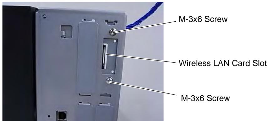
6. Attach the Antenna Cover to the printer back with the two M-3x6 screws, as shown below.
