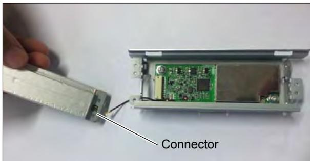
1. After the antenna shield and antenna screws have been removed, detach the connector of the PCB from the antenna.
