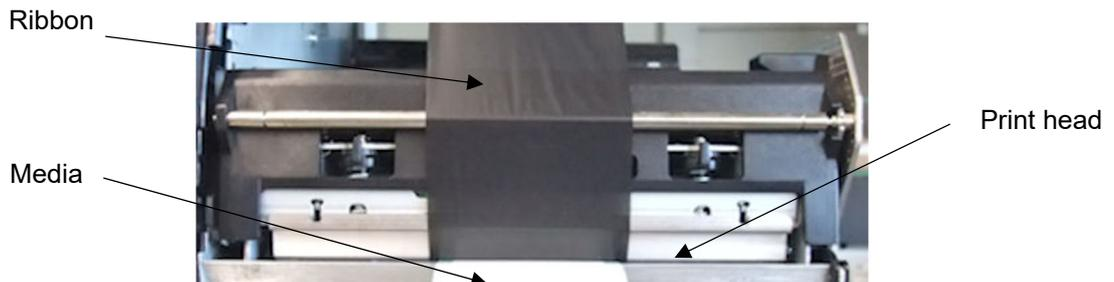
Ribbon wrinkle problem tends to occur depending on the various conditions, such as ribbon width, media width, ribbon motor torque, and print head position.
