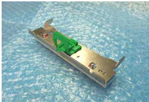
**Note 1:** Be sure to place the print head on a soft cloth or antistatic sheet.
