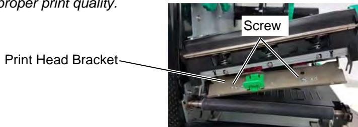
4. Never disassemble the head block frame. Doing so may cause a print failure, such as ribbon wrinkle, blurred print, etc.
