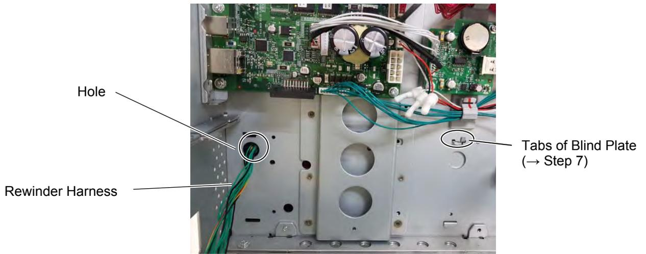
5. Pull out the Rewinder Harness from the opposite side, and re-connect it to CN1 on the Rewinder PC Board.
