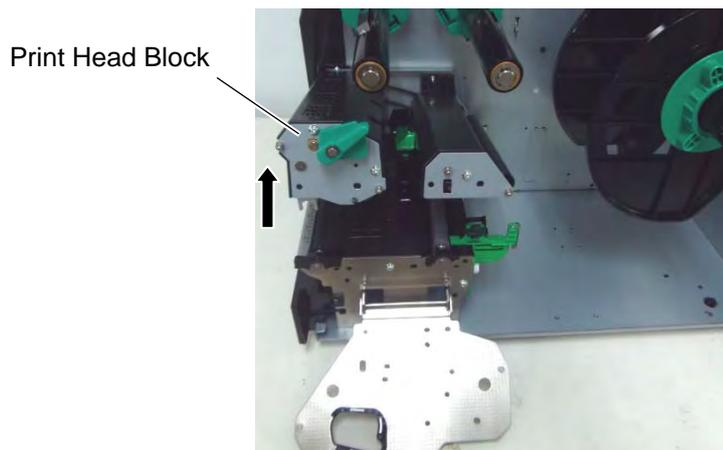
**NOTE:** DO NOT excessively push down the print head block to close it. Doing so may cause a failure of the print head block or damage to the print head.
