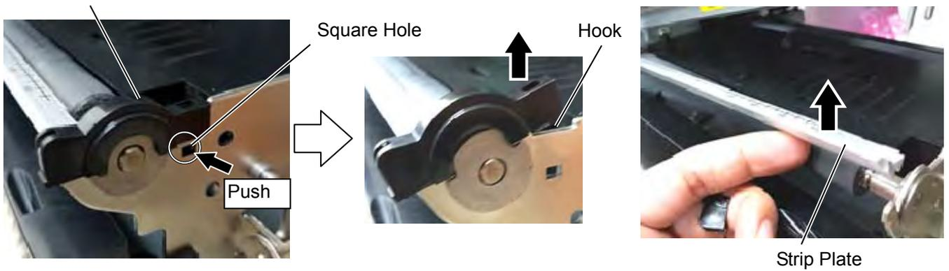
4. Install the RFID paper guide and return the platen holder cover to the original position.
