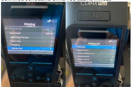
HIT THE ENTER BUTTON, SCROLL TO CALIBRATE AND HIT THE ENTER BUTTON, SCROLL TO AUTO CALIBRATION HIT THE ENTER BUTTON, SCROLL TO I-MARK AND HIT THE ENTER BUTTON
