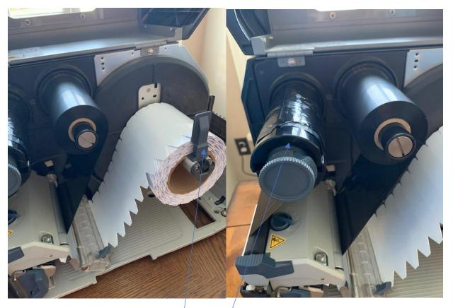
THE RIBBON SUPPLIED IS COATED SIDE OUT AND WILL BE INSTALLED AS SHOWN ABOVE
