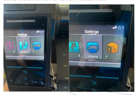
SCROLL TO THE LEFT TO GET THE PRINTING USING THE ARROW ENTER PRINTING BY USING THE ENTER BUTTON
